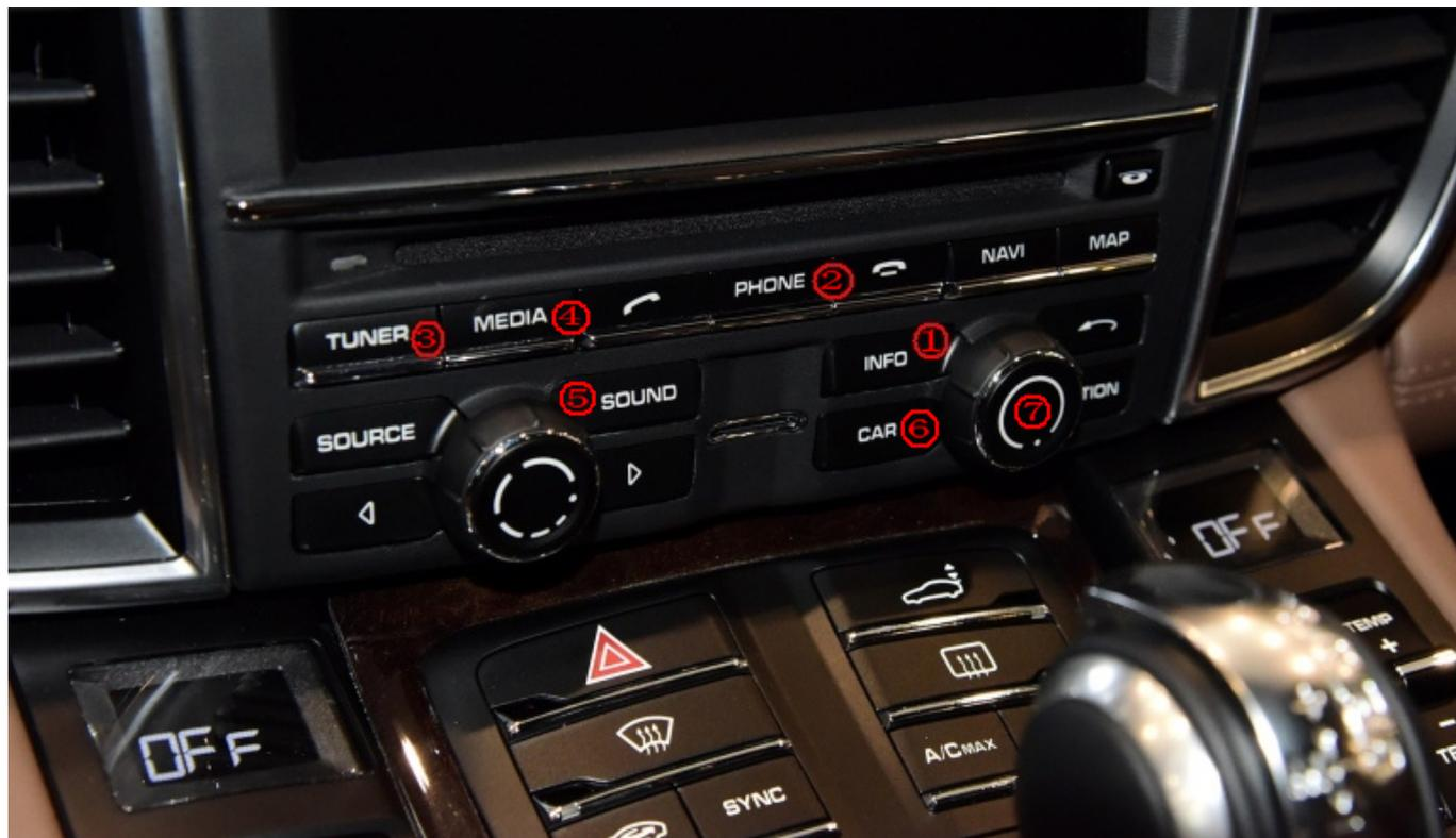
**3-1.①②**:长按其中任何一个键 3 秒可以在原车和解码器界面切换/Long press any key of them for 3 seconds to switch between the original vehicle and the decoder interface
